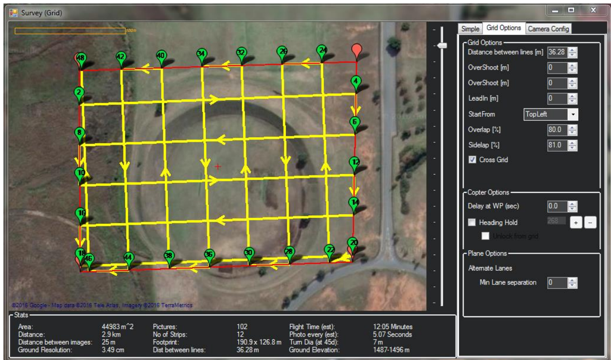
Figure 5: Screenshot of automatic flight plan generation in software tool
