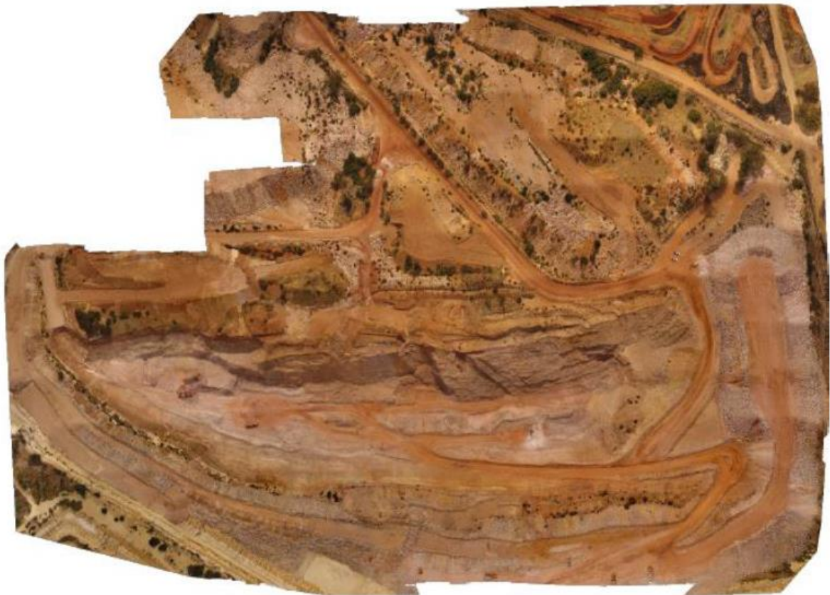
Figure 18: Geo-referenced orthomosaic map from of aerial image dataset (example: mining pit)
