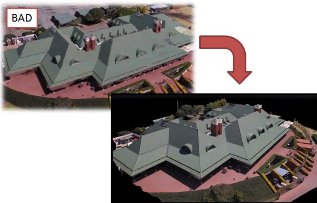
Figure 17: Point cloud filtering and sanitation process to improve quality of more detailed area.
