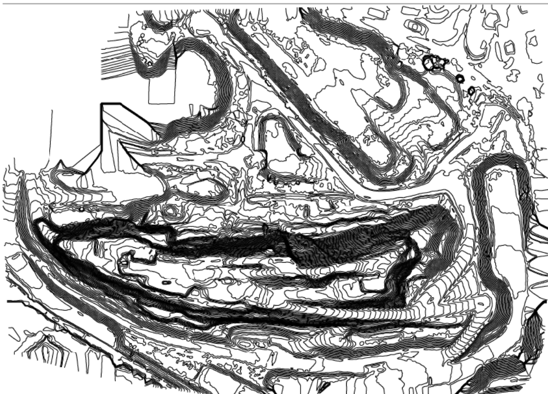
Figure 20: Contour line map, created from reconstructed 3D terrain (example: mining pit)
