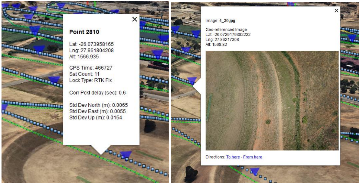
Figure 8: Flight and measurement data (currently geo-referenced images) displayed in Google Earth environment by clicking on respective objects in projected flight path.
