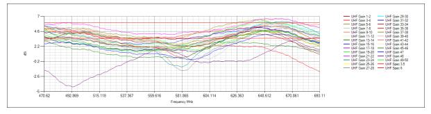
From the measured results and the quoted gain figures we can produce statistics that states the standard deviation and gain variance of the performance for the batch of antennas. The gain specified for the antenna gain curves above is between 3.5 dBi and 6 dBi. It can clearly be seen that the antenna does not reach the specification.
