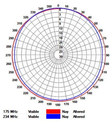
Antenna elevation pattern for two frequencies
